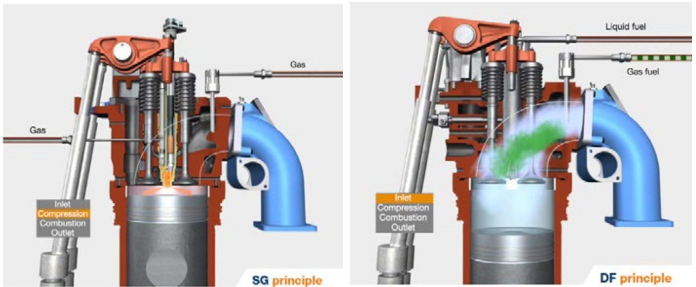
Figure 2: Wärtsilä 31 engine in spark gas (SG, left) and dual fuel (DF, right) versions.
