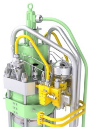
Figure 1: Cylinder cover with dual fuel LPG-diesel injection system on the MAN ME-LGIP engine.
