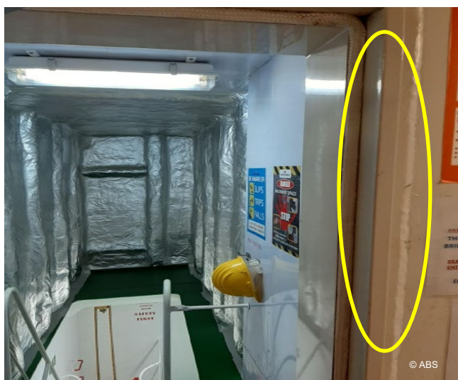
Engine room door gasket worn
