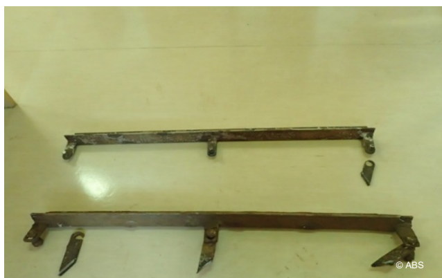
Fire damper broken linkage – before repair
