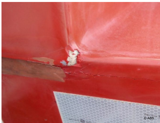
Rescue boat – hull cracks
