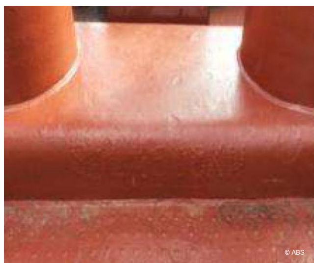
Mooring bitt not marked with SWL in contrasting color – before
