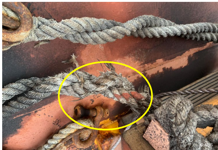
Embarkation ladder side rope rotten and broken
