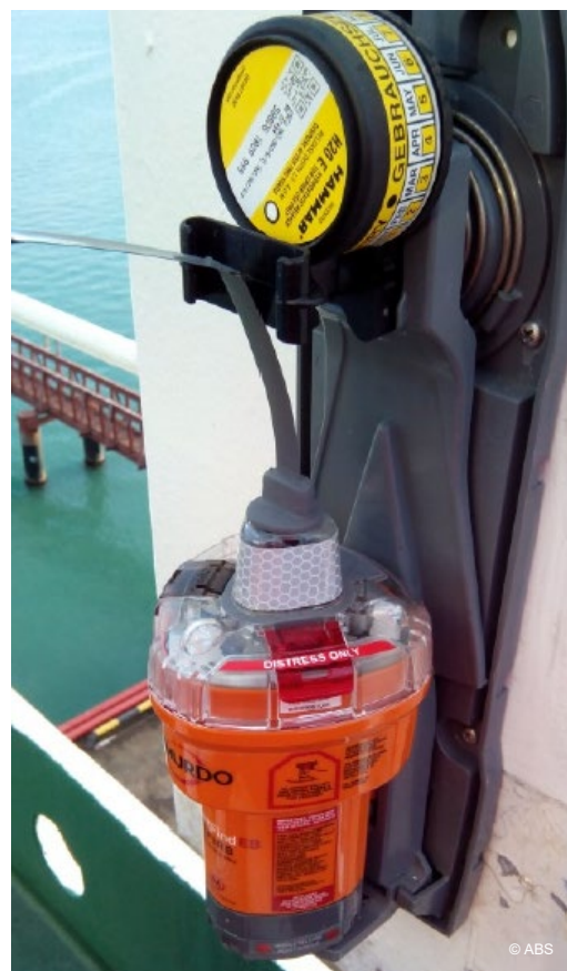
EPIRB antenna found deformed
