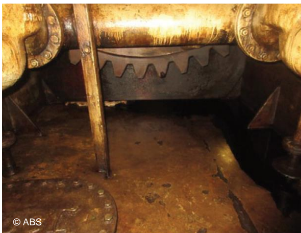
Oily bilges create fire hazards
