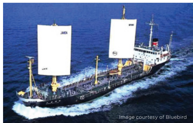
Vessel Shin Aitoku Maru with rigid sails
